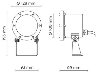
**! THIS LUMINAIRE IS SUITABLE ONLY FOR UNDERWATER INSTALLATION**
